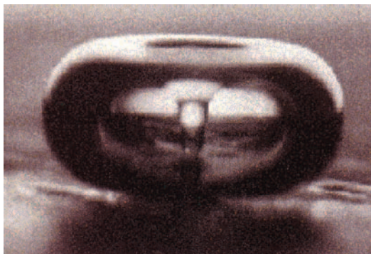
Figure 38-20 Image of a cavitation bubble collapsing on a metal surface. A jet of fluid can be seen punching through the center of the bubble toward the metal surface. Reproduced with permission from Crum LA. 27
